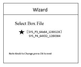
Note: The box files need to be imported into the equipment through the upper computer software.
