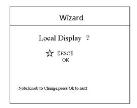
Note: This interface is to select whether it is necessary to intercept part of the image of the input signal source and display it on the LED screen.
