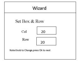
Note: Number of rows/columns in the box refers to the number of horizontal/vertical receiving cards used in the large screen.
